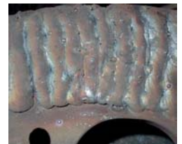
These weld beads will yield a nice set of slots. For a solid rotor, flow the beads together a for a flatter surface.
