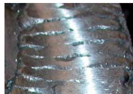
The final surface. The "slots" left in the surface will allow gases to escape to ensure a solid interface between the pad and rotor. This rotor is ready for another season!
