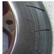
One season of light use. This rotor is not ready for the scap heap yet.
